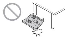
Hold the standard input tray with both hands when removing or installing. The standard input tray weighs approximately 2.9 kg (6.4 lb) when the recording paper is fully loaded.
